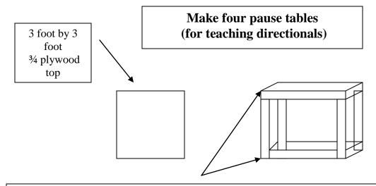
Approx. 20 inches tall 2 inch PVC Pipe box frame, top screwed on with deck screws
